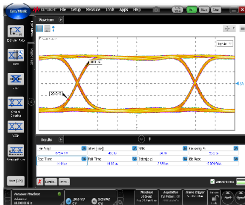
Input signal Eye amplitude = 0.66\text{ V}_{pp}
